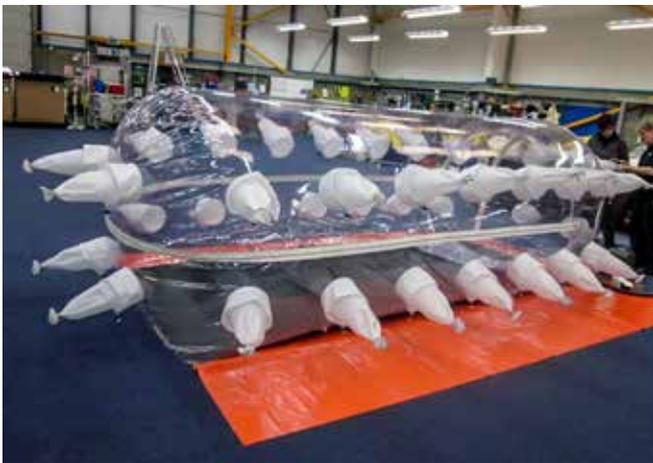
*Fig. 5. Multi-access enclosure manufactured to allow for several smaller fabrications to be welded in the same gas cycle. Alternatively, it can also be used for a single large item requiring access to several joints. Simultaneous multiple training can be undertaken.*
