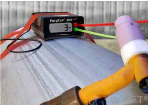
*Fig 3 Providing a sealed volume below the joint and purging with inert gas goes a long way to preventing oxidation. However, the purge gas itself need to be continuously monitored to ensure that a low oxygen content is maintained. This can be undertaken by using a monitor capable of detecting very low levels of oxygen. Advanced instruments such as the PurgEye range from Huntingdon Fusion Techniques meet these requirements.*
