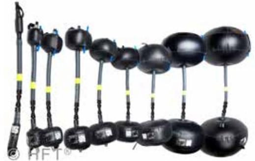
*Fig 2 A family of integrated purge systems is available covering all tube diameters from 25 mm. These offer total protection against oxidation during welding by providing a purge gas oxygen content as low as 10 ppm*
