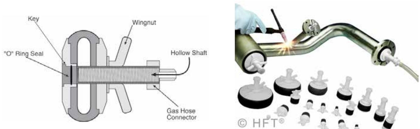
Fig 1 Tube diameters from 15 mm can be purged effectively using this type of engineered plug. Inert gas passed in at one end can be analysed for oxygen level at the exit.
