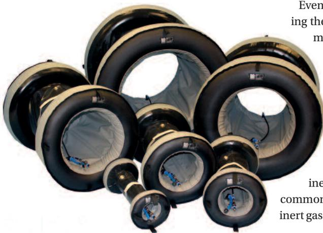
Flexible ‘floppy’ discs connected by a flexible tube are available. They can be deployed quickly and the removal after welding is easy since the assembly can be withdrawn past the weld. The reliability is suspect, however, because a disc to pipe sealing depends upon a very small contact area. Some have a semi-rigid connecting tube and this may be unsuitable where the system needs to be used either side of a sharp pipe bend. The working range of these systems is also very low.
