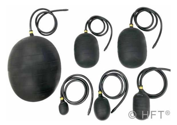
HFT® Rubber PetroChem Stoppers are for line pipe applications. Each Stopper has a longer length than diameter, which prevents them from tipping over inside the pipe and losing their seal. They also have a ribbing to prevent slipping.
