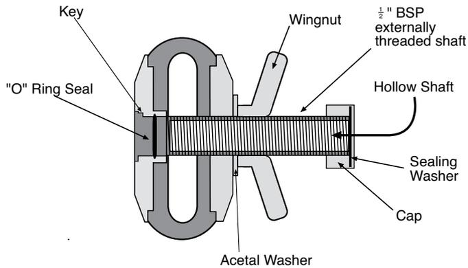
As can be seen from the sectioned view, the unique assembly of the central waterway into the base plate via a snap taper fit and "O" ring seal provides a positive water and air tight joint. The provision of a friction reducing acetal copolymer thrust washer inserted between the wing nut and top plate facilitates easy expansion and release.
