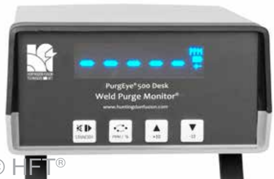
PurgEye® 500 Desk with PurgeNet™ similar to the PurgEye® 300 Plus but with an integral pump to take samples of exhaust gas at regular time intervals to be set by the user. Measuring range 1,000 to 10 ppm oxygen.
