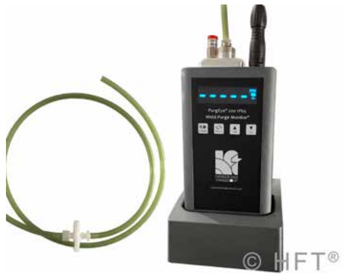
PurgEye® 200 IP65 Hand Held with PurgeNet™ new battery powered with an Integral sampling pump to drag samples across the sensor at regular, predetermined intervals. Measures down to 10 ppm oxygen. This model is also sealed against the ingress of water and dust, up to IP65 standard.
