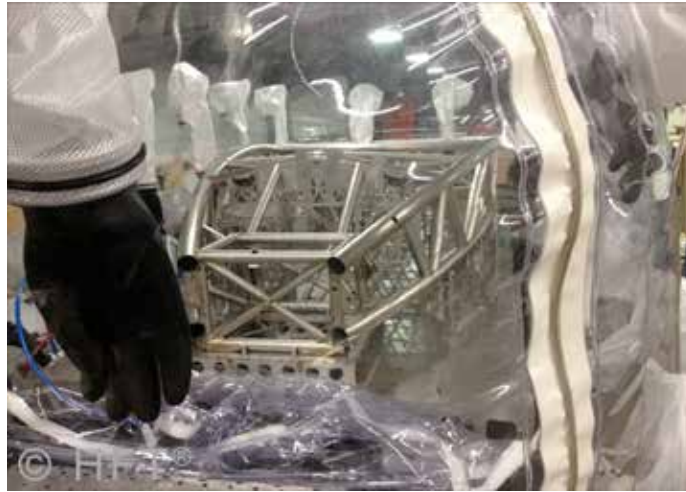
Titanium structure welded in an enclosure to provide bright shiny welds free of oxide discoloration.
