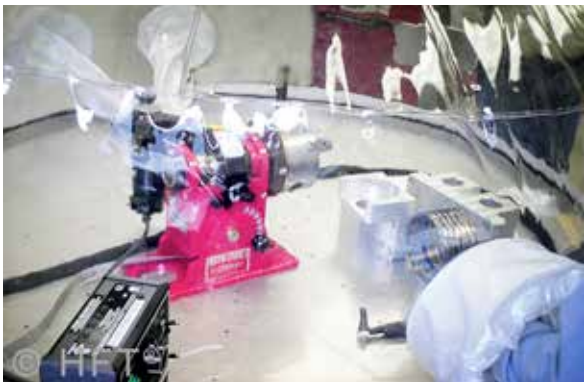
Welding titanium and other sensitive materials successfully requires an entirely clean and draught free work area
