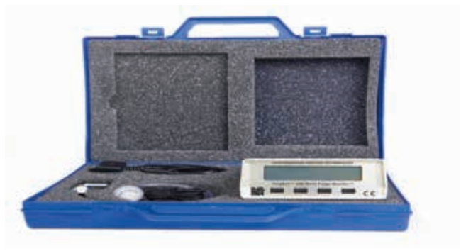
Figure 3. PurgEye monitors have been specifically designed for indicating oxygen levels in inert gas during weld purging. These rugged instruments have a measuring range down to 1 ppm on an alpha-numeric display.
